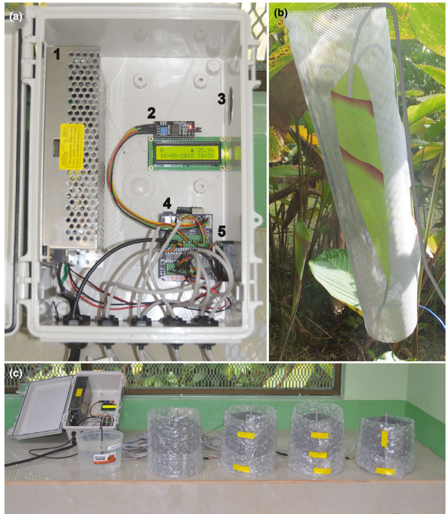
FIGURE 2 Heater implementation. (a) Heater control box, containing a DC power source (1), LCD (2), air outlet (3), heater control shield and Arduino UNO microcontroller board (4), air intake with fan (5). See Figure 1 for control shield wiring details. (b) Heater (powered by the blue wire) with temperature sensor (grey wire) on a rolled leaf. This image is a composite of a photo and digital drawings, as the leaf inside the heater and the temperature sensor wire are otherwise very difficult to see. (c) Heating 2-L aquatic microcosms in an ambient laboratory. Heater screens (grey) are wrapped around plastic containers and insulated with a layer of bubble wrap. The control microcosm is on the far left
